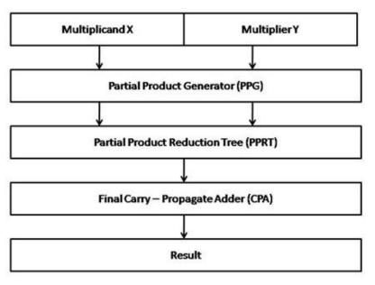
Fig. 4: Block diagram of Modified Booth multiplication process.
