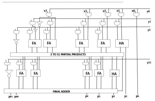
Fig. 2: 32-bit array multiplier [63]
