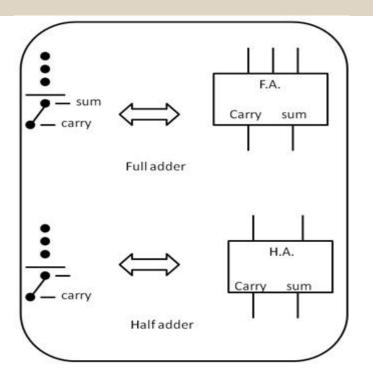
Fig. 6: Representation of half adder and fulladder
