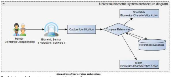
Fig. 3: Universal biometrics system architecture diagram.
