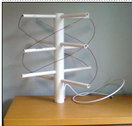
Fig. 8: Experimental Sample of the QHA . Antenna – Courtesy of Manual: by Ilcev [4]
