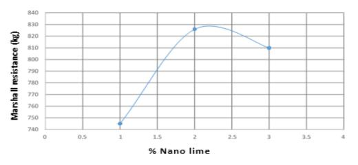
Fig.6: Marshall Resistance changes - the percentage of Nano Lime
