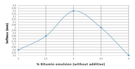
Fig. 4: The softness changes - the percentage of bitumen emulsion (without additives).
