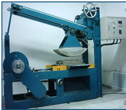
Fig: 2. Roller compactor machine
