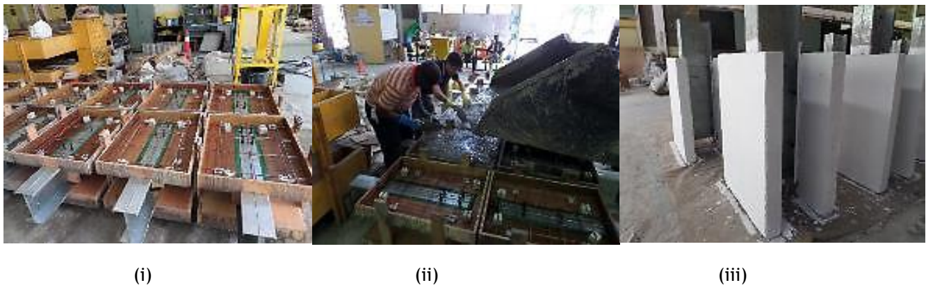
Fig. 1: Preparation of test specimens (i) Formwork, (ii) Casting, (iii) Finished samples
