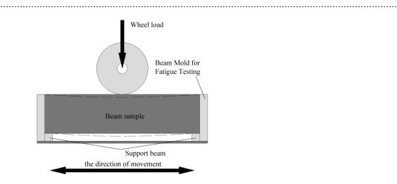
Fig. 4: Sample load for PT fatigue test method.
