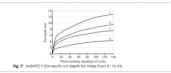
According to AASHTO TP 63, the allowable rut depth should be no more than 12 mm after 8000 wheel cycles. For the control specimen such rut depth has reached after the 7800 wheel cycles. For the SEA such rut depth does not reached even after the 10000 wheel cycles; the maximum depths are 7.38, 5 58 and 3.64 mm for the mixes 2–4, respectively.
