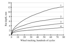
Fig. 6: AASHTO TP 63 results: rut depth for mixes from #1 to #4.
