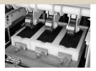
Fig. 3: Experimental setup for PT fatigue test method.
