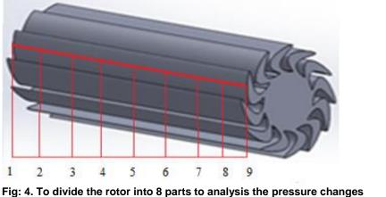
At first, the bladder-formed rotor, the changes of pressure in bladdered rotor surface is shown in the purposed points in **Table-1**.
