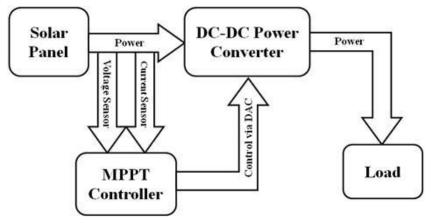
Fig. 2: Block diagram of MPPT [4]
