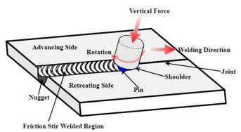
Fig. 1: Schematic drawing of the FSW technique [9].
