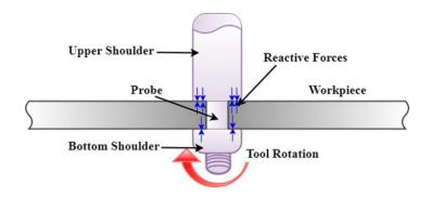
Fig. 2: Schematic of self-reactive or bobbin tool FSW [14].
