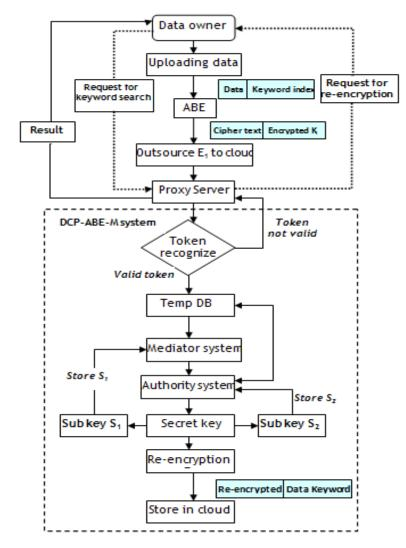
Fig. 3: Flow chart for DCP-ABE-M-ABPKS system processing.
