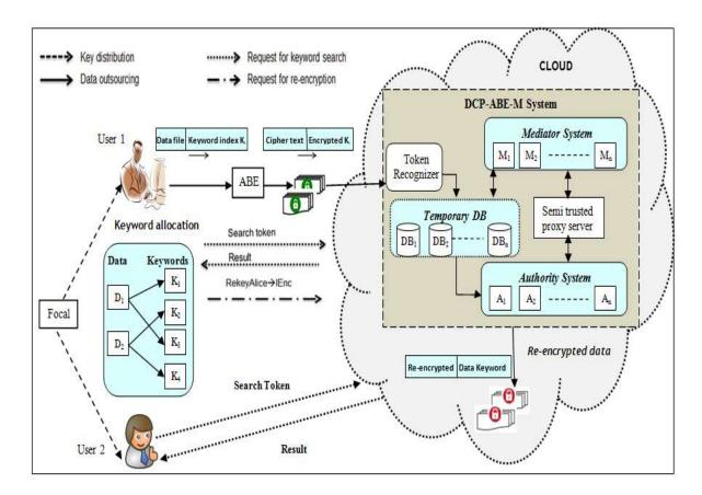
Fig. 2: Architecture of DCP-ABE-M-ABRKS system.
