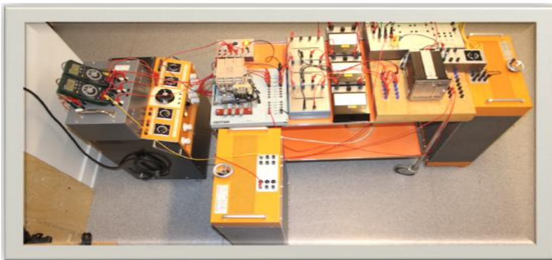
Fig: 18. Phase to Earth Network with resistance grounded neutral (Earth Fault Circuit)
