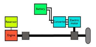
Fig. 1: Simplified structure of a combined hybrid electric vehicle
