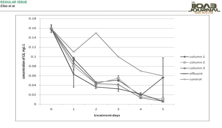
Fig: 7. Cadmium removal profile in each column during the treatment of ceramic wastewater using water hyacinth
