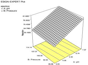
Fig: 5. Response surface plotting for the effect of controlled parameters on glucose removal efficiency
