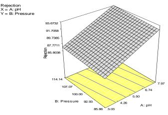
Fig: 3. Surface response plot for the effect of controlled parameters on DDT removal efficiency (relationship between operating pressure, pH and DDT removal efficiency)
