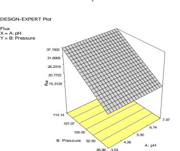
Fig: 2. Surface response plot (relationship between operating pressure, pH and permeate flux for DDT)
