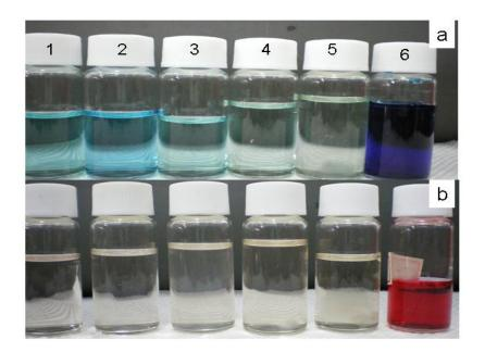
**Supplementary Figure (IIa)** No. 1- 1.0 g of unmodified sludge; No. (2 - 5) - 1.0 g - 4.0 g of modified sludge; No, 6- methylene blue solution (100 mg L<sup>-1</sup>) (**IIb**) No. 1- 1.0 g of unmodified sludge; No. 2- 5-1.0 g - 4.0 g of modified sludge; 6-Acid red 114 (100 mg L<sup>-1</sup>)
