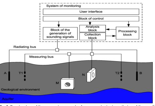
Fig. 1: The structure of the measuring complex for geoecological monitoring of the aquifer.
