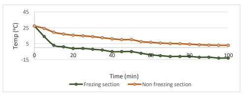
Fig. 5: the temperature distribution in the evaporator over time.
