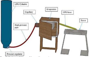
Fig. 2: Setup of the refrigeration system.
