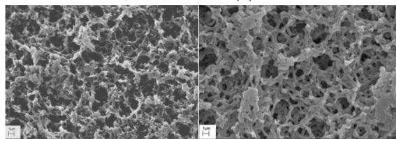
Fig. 3: Image of the surface of the original (left) and microwave treated in air (right) membrane with 3000x magnification.
