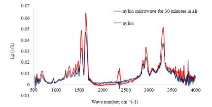
Fig. 2: IR absorption spectra of nylon before and after treatment with microwave radiation in an air environment for 30 minutes.
