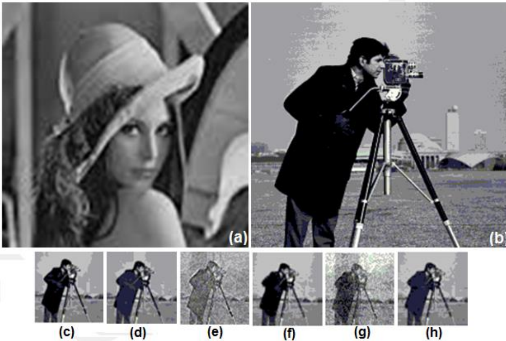
Fig: 3. (a) Original image, (b) watermark, (c) Extracted watermarks after cropping, (d) Rotation, (e) Gaussian noise, (f) Average filtering, (g) Histogram equalization and (h) JPEG compression attacks respectively
